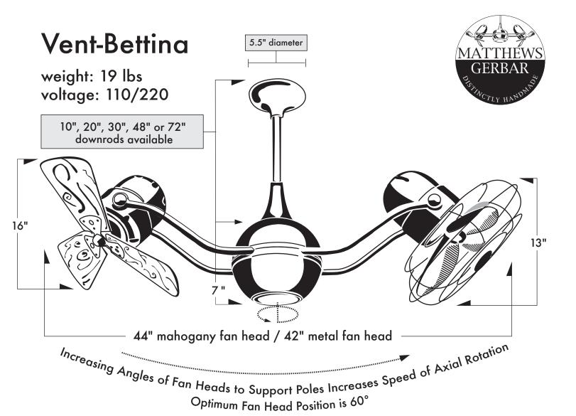
CFM: 4240 (Wood Fan Head) Blade Pitch 19° CFM: 3201 (Metal Fan Head) Blade Pitch 31°
