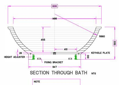
KEYHOLE PLATES CAN BE USED AS DEMOUNTABLE FIXINGS BETWEEN BATH AND PLINTH TO ENABLE PLINTH TO BE ANCHORED TO FLOOR HELIO BATH DATA SHEET
