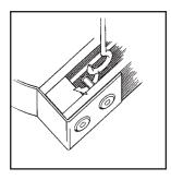
NOTE: If the rack isn't level, unhook the extension hook from the incorrect corner. Adjust the ceiling screw by turning it 1/2 turn in the appropriate direction. Reinsert the extension hook.
