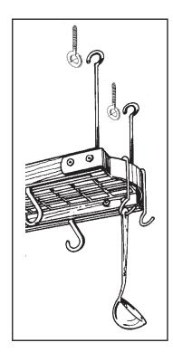
The screw eyes *must* be securely installed into solid wood. Sheet-rock fasteners will not hold enough weight and should not be used.
