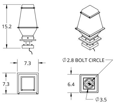
Mounting Method: Mounts Directly to Pier
